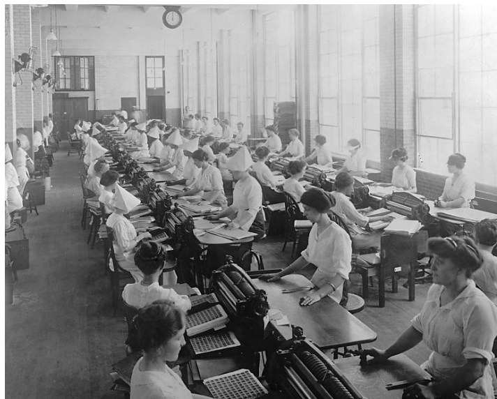
Figure 6.15. Perforating stamps, using 46 machines (total capacity of 105,000 sheets/day), 1914. Courtesy The Library of Congress, LC-DIG-npcc-31460.
